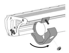
5. Lightly fasten light bar to tube by attaching supplied ARB M6 security nuts to T-bolts. Adjust rotation of light bar on tube to appropriate position and tighten security nuts using security key provided to 9 Nm / 80 lb-in.
